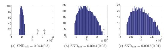
**Figure 14.** Eigenvalue histograms of reconstructed covariance matrix in the three-class case for three SNR values. Note that the noise distribution initially engulfs the second eigenvalue, and eventually the top eigenvalue as well.
