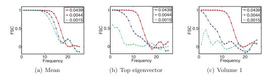
**Figure 10.** FSC curves for the mean volume, top eigenvector, and one mean-subtracted volume at the same three SNRs as in Figure 8. Note that the mean volume is reconstructed successfully for all three SNR levels. On the other hand, the top eigenvector and volume are recovered at the highest two SNR levels but not at the lowest SNR.
