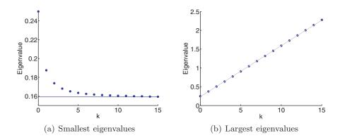
**Figure 6.** The smallest and largest eigenvalues of (the continuous version of)  $\hat{L}^{k,k}$ , for  $0 \le k \le 15$ . The smallest eigenvalues approach their theoretical lower bound of  $1/2\pi$  as k increases. The largest eigenvalues show a clear linear dependence on k.
