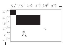
**Figure 5.** Block diagonal structure of  $\hat{P}_s$ . The shaded rectangles represent the nonzero entries. For an explanation of the specific pairing of angular and radial functions, see (5.27) and (5.19) and the preceding discussion. A short calculation shows that the kth block of  $\hat{P}_s$  has size  $(k+1) \times \frac{(k+1)(k+2)}{2}$ .
