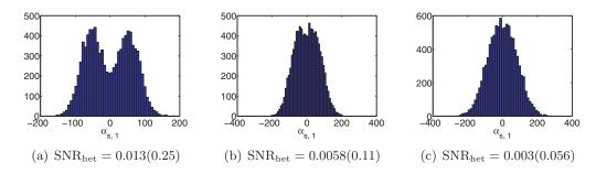
**Figure 12.** Histograms of  $\alpha_s$  for two-class case. Note that (a) has a bimodal distribution corresponding to two heterogeneity classes, but these two distributions merge as SNR decreases.
